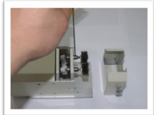
2. Remove the set screw.
