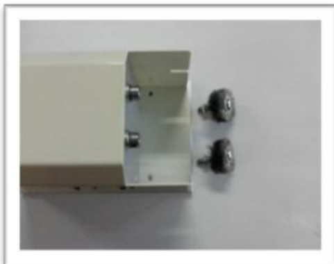
5. Screw the fixed hexagon wrench and take off the brushes.
